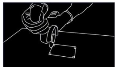
making L-shape and angled cuts on porcelain tiles with cnc or water-jet machines and even manual. that should make rounded-off edge to protect the tiles from breaking.
