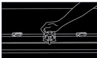
cutting machines have holders to fix the tiles during cutting process. and also some manual strong holders should be used to fix the edges of two tiles together.
